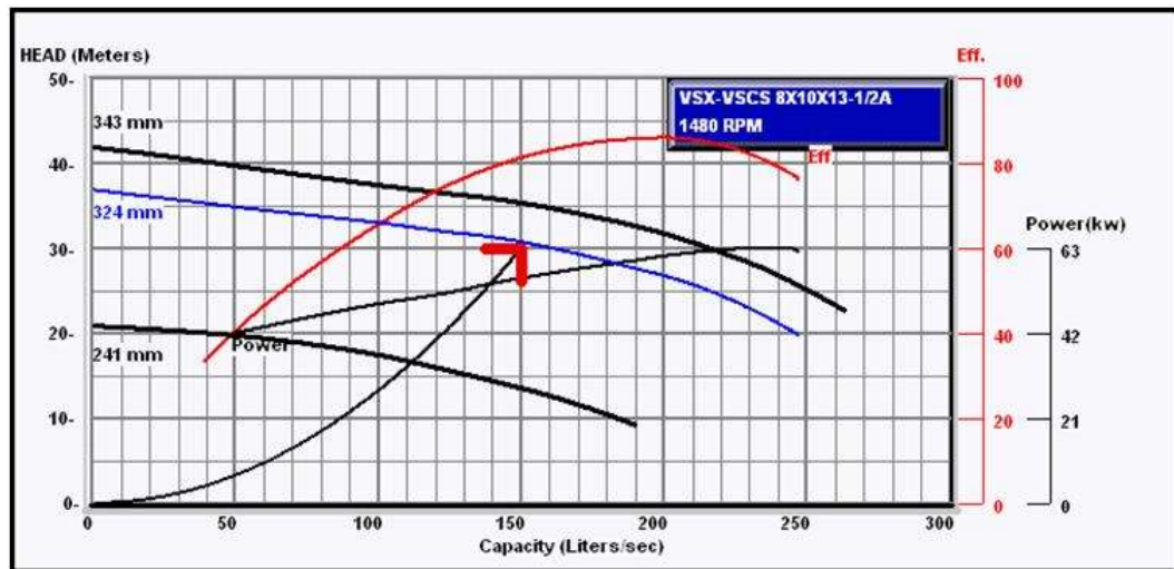
Figure 5.27 Pump operating point for pump sized for 50% of the capacity (courtesy of ITT Bell & Gossette ESP-Plus pump selection software)
