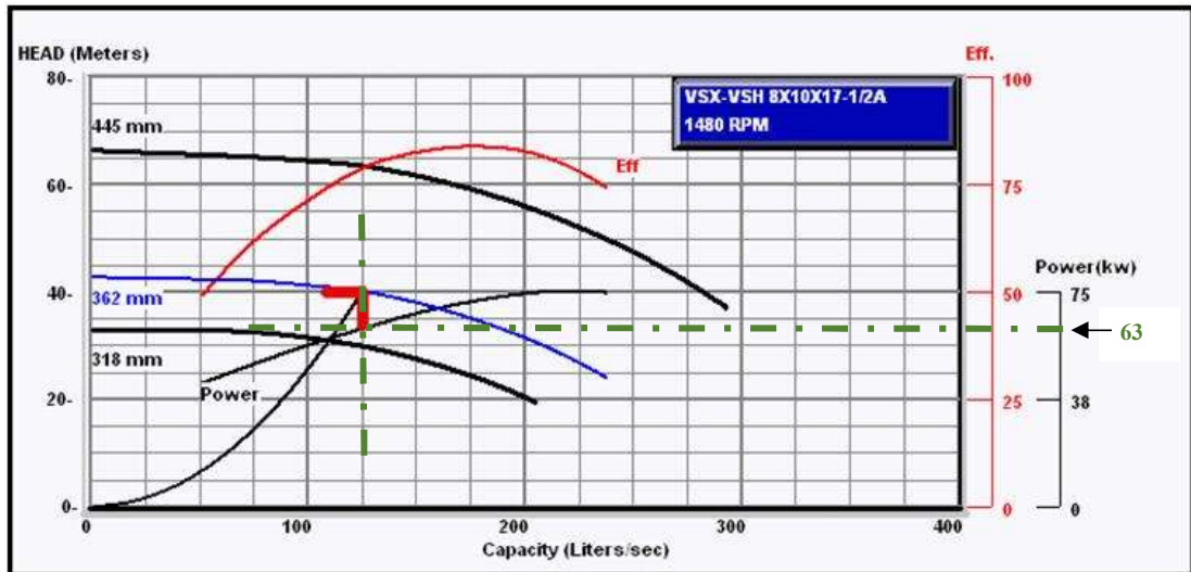
Figure 5.25 Pump operating point for a pump operating at 1480 rpm (courtesy of ITT Bell & Gossette ESP-Plus pump selection software)
